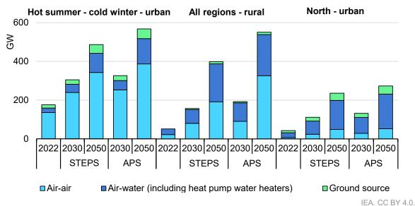
The installed capacity of heat pumps in China increases in all climate zones in the STEPS and APS.
