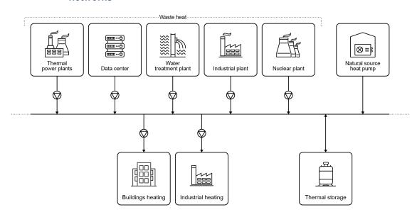
Figure 2.7 The integration of heat pumps and waste heat in district heating networks
